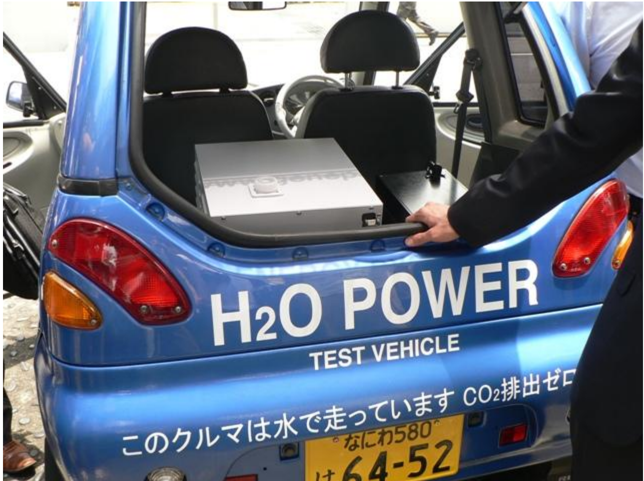
300W generation system mounted in a luggage room (left) teck-on
